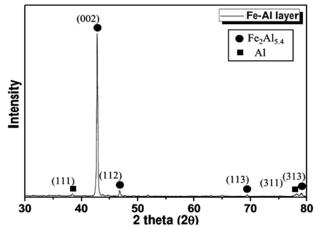
Figure 5: XRD Result Around the Point a
