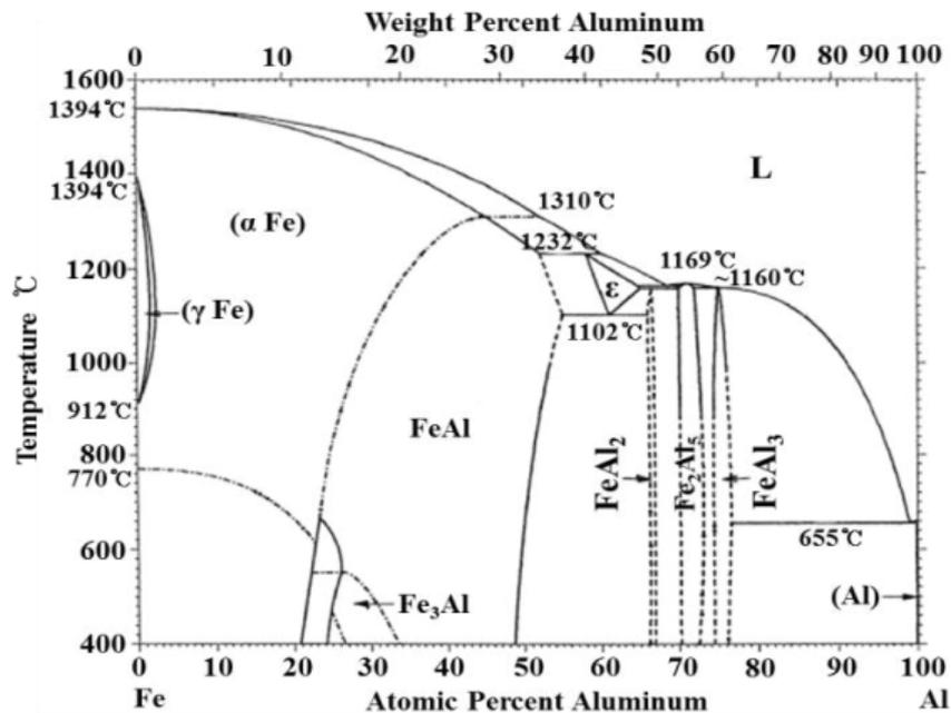
Figure 9: Binary Phase diagrams of Fe-Al
