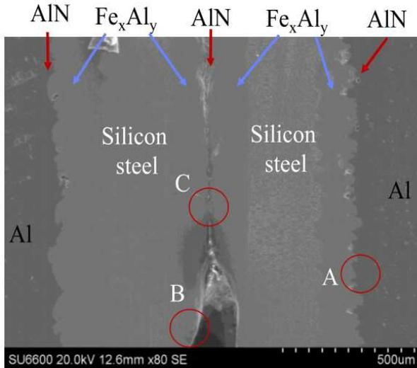
Figure 2: SEM Image of the Silicon Steel-Al Plate Multilayer
