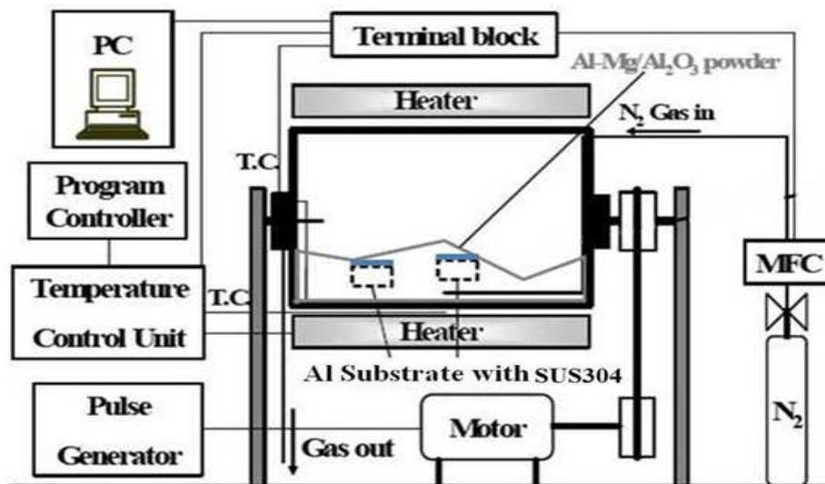
Figure 1: A Schematic Diagram of the Barrel Nitriding Process
