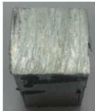
Figure 8: Photomicrograph of Worn Surface of 3 wt.% TiC/7075 Composite at 1140 rpm and Load 20 N after 10 Min
