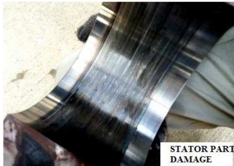
Figure 2: Stator Part Damage Due to Seizure
