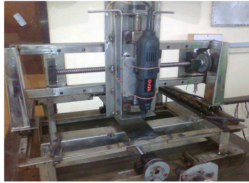
Figure 4: Partial Assembly of the Router
