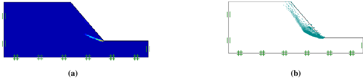
Figure 10: Shear Strains and Area Displacement by \alpha_2 = 55^\circ
