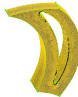
Figure 4: RCV Grid Set Up
